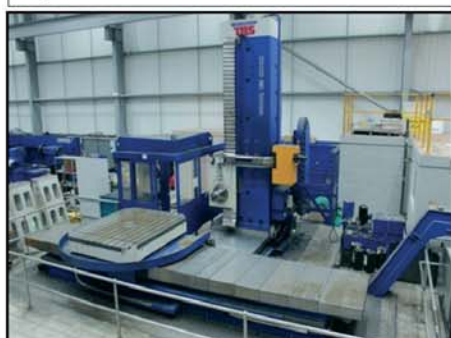
CNC-5-axis horizontal Table Type Borer TOS VARNSDORF WHN(Q) 13 CNC , built 2015, SIEMENS 840 D solution line, XYZWB 4.000x2.500x1.250x800 mm 360°, 37 kW
