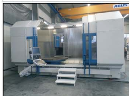
5-axis-CNC-Machining Centre AXA VHC 3-XTS/50 , retrof.2016, HEIDENHAIN iTNC 530, XYZ 2.600x900x850 mm, NC-rotary table 1.500 mm, 56 kW, 30-9.000 min -1 , 60 ATC
