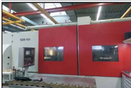
CNC-Turning- Milling Centre MAG NDM 450-4-300 , built 2008, SINUMERIK 840D, turning \varnothing 450 x 3.000 mm, 95 kW, subspindel, B-axis, Y-axis, milling spindle
