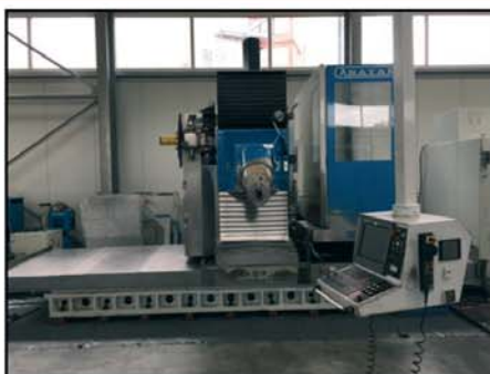
CNC-Bed Milling Machine ANAYAK HVM 3300 , built 1998, HEIDENHAIN TNC 426, XYZ 2.700x1.200x1.000 mm, ISO 50, 30 kW, 20-4.000 min -1 , 40 ATC
