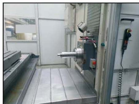
CNC-Horiz. Boring-Milling Machine UNION TC 110 , built 2014, HEIDENHAIN iTNC 530 HSCI, quill \varnothing 110 mm, 4.000 min -1 , 22/27 kW, X-Y-Z-W 1.500x1.250x1.000x550
