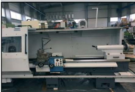
CNC cycle-controlled Lathe WEILER E 70 , built 1998/2017, SINUMERIK 810D, turning length 2.000 mm, machine geometric overhauled
