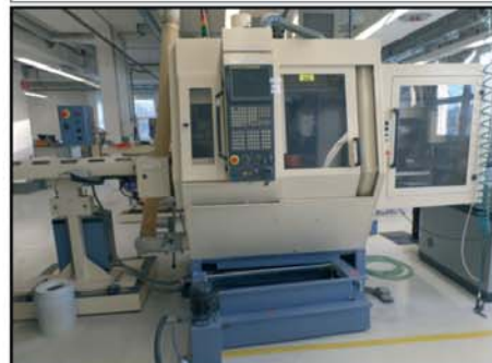
5-axis-CNC-milling center WILLEMIN W 408 MT , built 2006, GE FANUC Series 161-MB, 24-fold tool changer, workpiece handling
