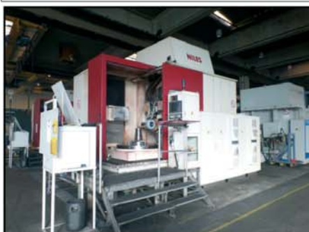
CNC-Gear Grinding Machine NILES ZP 20 , built 2006, SINUMERIK 840 D, max. \varnothing 2.000 mm, max. profile depth 75 mm, max. module 34 mm, internal grinding device
