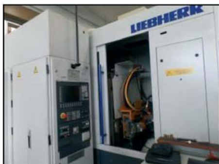
CNC-Gear Hobbing Machine LIEBHERR LC 150 , built 2004, SIEMENS 840D, max. workpiece \varnothing 150 mm, ring loader
