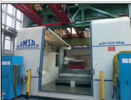
CNC-Deep-Hole-Boring- and Milling Machine IMSA MF 2500 BB , built 2012, HEIDENHAIN iTNC 530, X-3.300 mm, workpiece table 2.500x2.000 mm
