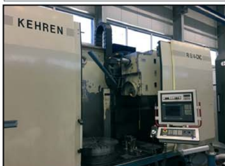
CNC-Rotary-Grinding Machine KEHREN Ri 8/4 CNC , built 1998, SINUMERIK 840 D, rotary/grinding \varnothing 800 mm, swing \varnothing 900 mm, 2 pc grinding spindles
