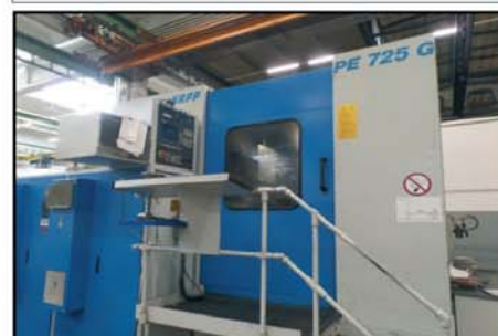
CNC-Gear Grinding Machine PFAUTER-KAPP PE 725 G , built 1996, SINUMERIK 840C, workpiece \varnothing 800 mm, NC-dresser, tailstock, coolant device
