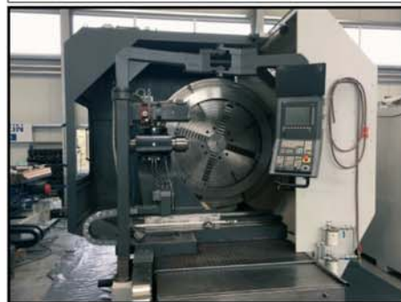
CNC-Facing Lathe GEMINIS GHT8-2200 , built 2012, SINUMERIK 840 D Shop Turn Power Line, \varnothing 2.200, 100 kW, C-axis, tool turret, face plate, milling unit
