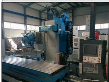
CNC-Bed Milling Machine ZAYER 20 KFU 4000 , built 2007, HEIDENHAIN iTNC 530, XYZ 3.700x1.200x1.500 mm, ISO 50, 28 kW, 35-3.000 min -1 , 30 ATC, 5.000 work hours
