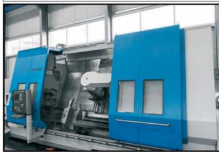
CNC-Turning-, Milling-, Boring Centre MAX MÜLLER MDW 20 M x 3.000 , built 2002, SINUMERIK 840C, \varnothing 850/690x2.960 mm, 56-3.000 min -1 , ATC 180, C-axis, tailstock
