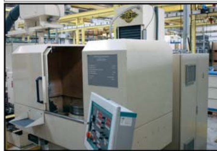
Rotary Table Surface Grinding Machine ELB ROTARY 60 S-H , built 1999, ELB-SPS control, table \varnothing 600/400 mm, load 300 kgs, 10 kW, 1.440 min -1
