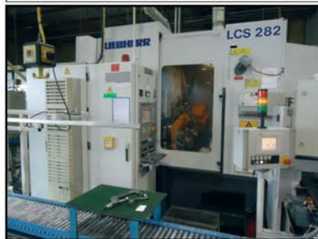
CNC-Gear Profile-Generating Grinding Machine LIEBHERR LCS 282 , built 2001, LIEBHERR-PC NC, max. wp. \varnothing 280 mm, min/ max. module 1/5 mm, 4-10.000 min -1
