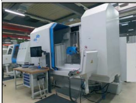
Precision Surface-Profile Grinder ABA POWERLINE 1004 , built 2009, 26 kW, SINUMERIK 840D, grind. LxW 1000x500 mm, table 800x400 mm, dresser, paper band filter
