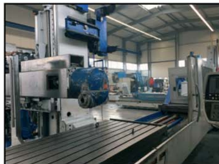
CNC-Bed Milling Machine SORALUCE TR 35 , built 2002, HEIDENHAIN TNC 430 M, XYZ 3.500x1.200x1.600 mm, ISO 50, 28 kW, 20-4.000 min -1 , 30 ATC
