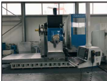
CNC-Bed Milling Machine ANAYAK HVM 3300 , built 1998, HEIDENHAIN TNC 426, XYZ 2.700x1.200x1.000 mm, ISO 50, 30 kW, 20-4.000 min -1 , 40 ATC
