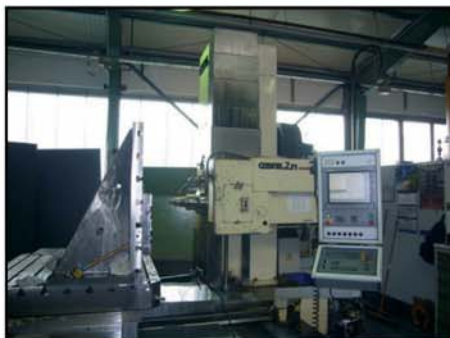
CNC-Horiz. Boring-Milling Machine CASTEL 2N , rebuilt 2005 HEIDENHAIN iTNC 530, quill \varnothing 100 mm, XYZW 2.000x1.500x 1.000x500 mm, NC-rotary table, 40 ATC
