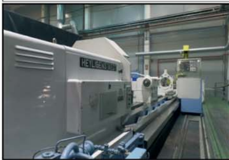
CNC-Heavy Duty Lathe HEYLIGENSTAEDT NDKb-800/III/16x6000 , retrofit 1996, \varnothing 1.580/1.280x6.000 mm, 2,8-340 min -1 , 63 kW, 3-bed guided, tailstock, tool turret
